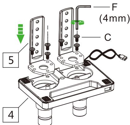
EN Thread the bolt in about 15mm.
