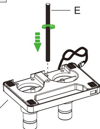
EN Thread the bolt in about 15mm.
